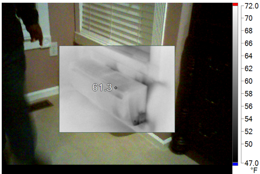
Thermal and air leak around room AC unit
